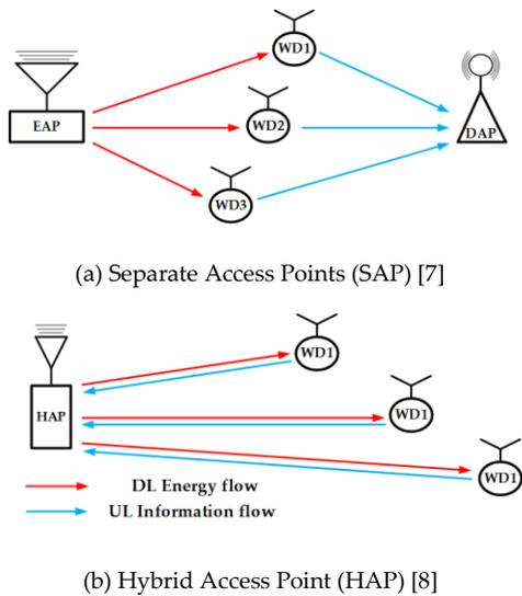
**Figure 1.** Wireless-Powered Communication Networks Model.
