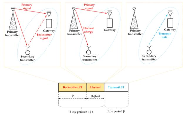
Figure 5. RF-Powered Backscatter Cognitive Radio Networks (CRN)
