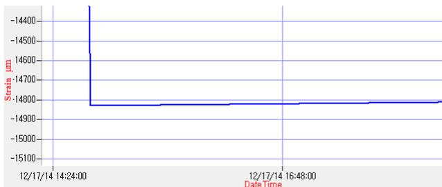
Figure 7. Output data of the “User Interface” software when the typical strain in cluding temperature sensed using the first (1/8) FBG sensor connected through channel 1/8
