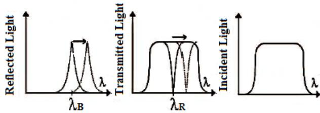
Figure 4. The comparison of Reflected, Transmitted and Incident Wavelengths in FBG sensor
