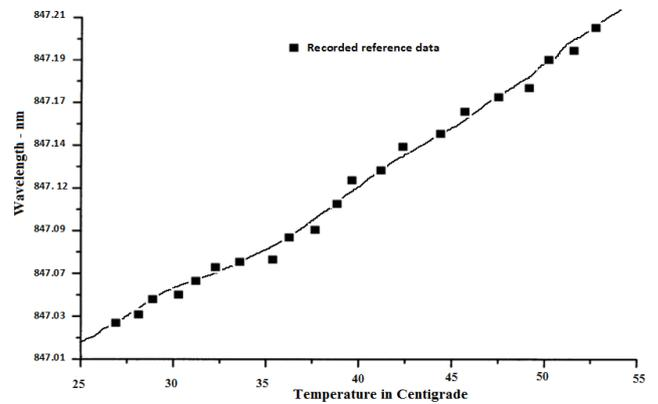
Figure 9. Typical comparison of the expert system output against FBG exposed to the temperature
