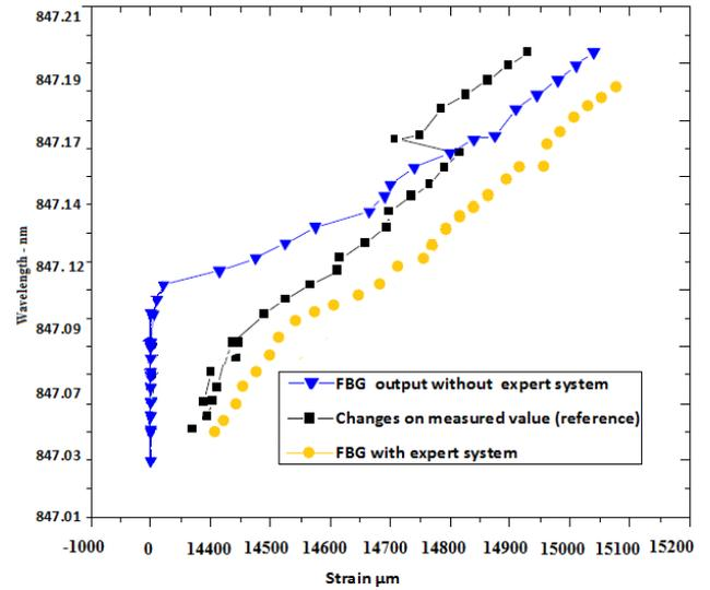
Figure 8. Typical comparison of the expert system output with direct FBG output
