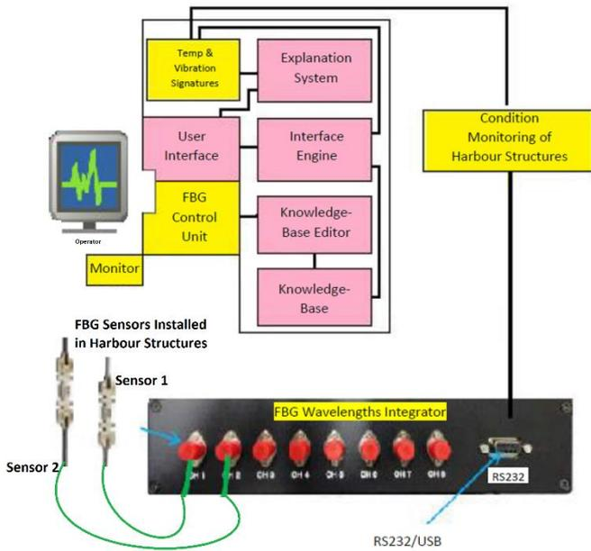
Figure 6. The most important FBG module of proposed rule-based expert system
