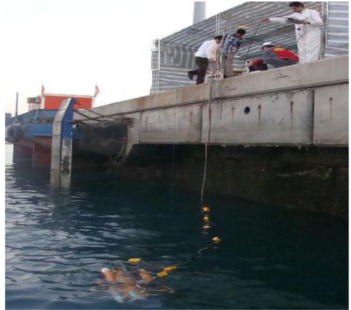
**Figure 2.** Localized vibration imposed to the quay wall using ROV based vibrator and receiving FBGs notification installed on the quay wall at Shahid Rajaei harbour
