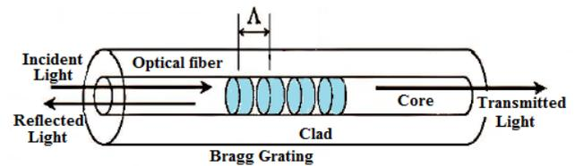
**Figure 3.** The interior structure of a FBG sensor
