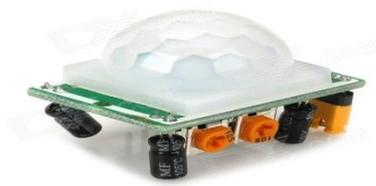
Figure 6. HC-SR501 movement sensor
