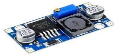
Figure 4. LM2596 DC/DC step-down voltage converter
