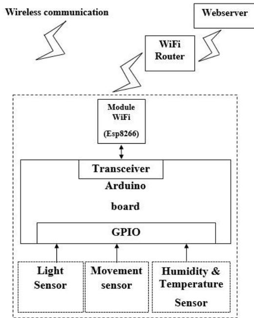
Figure 1. The system is model to be set up
