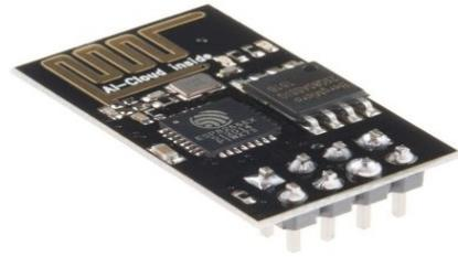
Figure 3. ESP-01 WiFi module with ESP8266
