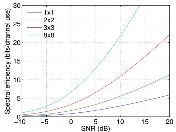
**Figure 2.** Spectrum efficiency via signal to noise ratio in a massive MIMO system with different antenna models. The greater the number of antennas, the more gain the system can achieve.
