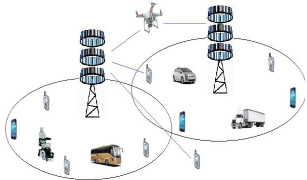
**Figure 1.** A massive MIMO system with cylindrical antenna array in wireless communication networks. The networks support many applications with different objects.
