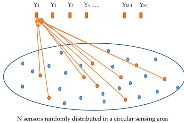
**Figure 2.** N sensors are deployed in a sensing area; only active sensors contribute to one CS measurement at a sampling time.
