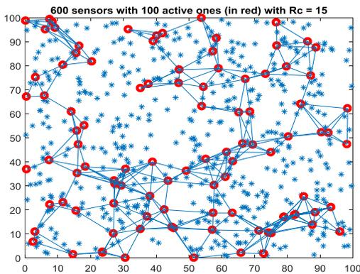
**Figure 1.** 600 sensors randomly deployed in a square sensing area 100\*100 unit square; 100 sensors are active and the communication range should be  $R_c = 15$  unit to be able to connect all active sensors.
