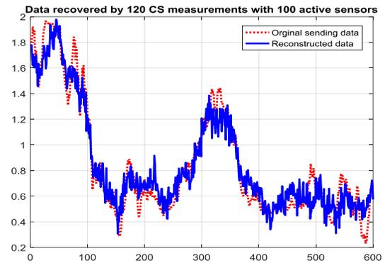
**Figure 3.** 100 active sensors create one CS measurements and whole reconstructed data recovered from 120 CS measurements
