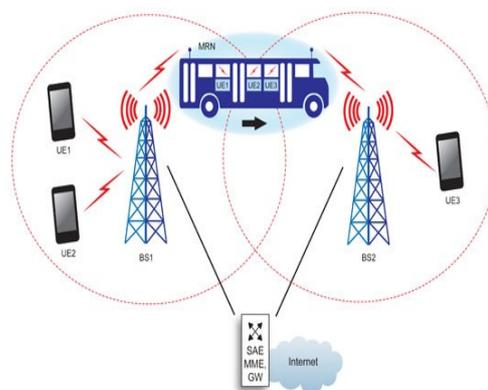
Figure 1. The basic structure of Wireless transmission
